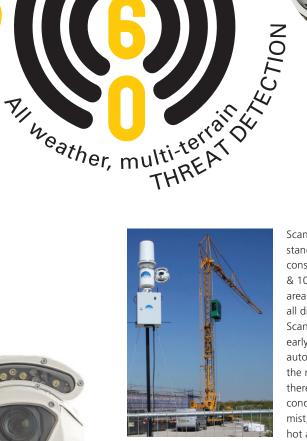
Scan-Integrated is a unique stand-alone intelligent system consisting of integrated Radar & 1080p HD Camera with wide area coverage of up to 200m in all direction (400m diameter). Scan-Integrated provides early warning detection and automatic surveillance without the need for visual clarity and therefore works in all weather conditions - rain, fog, snow, mist, coastal as well as extreme hot and cold climates.
