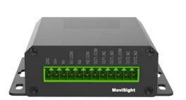
MS-7UC11 series LoRa wireless controller is a device used for data acquisition from multiple sensors. It contains different I/O interfaces including analog inputs, digital inputs, relay outputs, serial ports, which simplify the deployment and replacement of LoRaWAN<sup>®</sup> networks. Besides, MS-7UC11 series support multiple trigger conditions and actions which can work without network.
