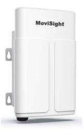
MS-7UG67 is a robust 8-channel outdoor LoRaWAN<sup>®</sup> hotspot, which is compatible with Helium LongFi technology. Adopting SX1302 LoRa chip, high-performance quad-core CPU and secure crypto chip, MS-7UG67 provides high-efficiency and reliable connection. MS-7UG67 has line of sight up to 15 km and can cover about 2 km in urbanized environment, which can cover larger areas and provide connectivity to more than 2000 nodes.
